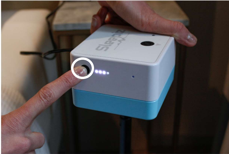
Figure 10. The battery status button is circled. Next to the button, there are 4 battery status indicators. When the battery is sufficiently charged to record for 8h, at least two battery status indicators turn on after the button press
