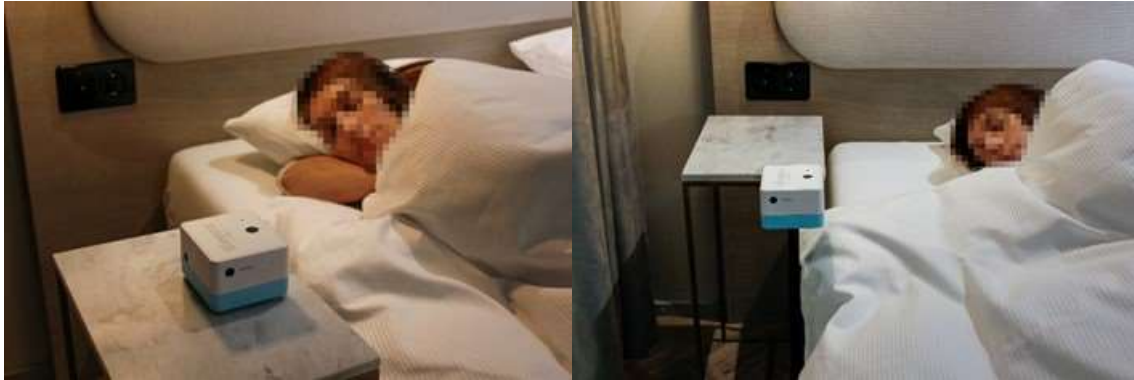
Figure 6. Alternative position of Sleepiz One+. A - on a bedside table, turned towards the chest; B - on the monopod
